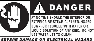
SEVERE DAMAGE OR ELECTRICAL HAZARI COULD RESULT. WARRANTY BECOMES VOID IF APPLIANCE IS FLOODED.
